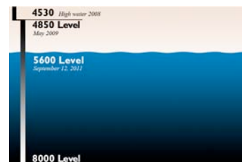
Figure 4: Progress of dewatering at Sanford Lab
