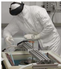
Figure 6: SDSMT grad student Mark Horton washes the surface of copper with deionized water to remove sulfate crystals in the MAJORANA temporary cleanroom
