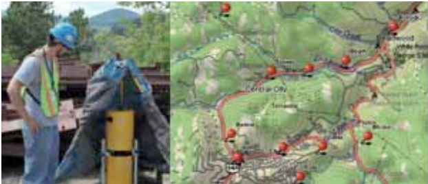
Figure 4: Left: USGS Research Hydrologist Andy Long checks gravimeter as it measures microgravity in the Ross Shaft yard. Map at right indicates measurement stations at or near Sanford Lab
