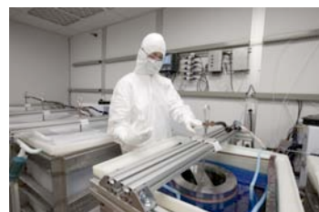
Figure 12: South Dakota School of Mines chemist Cabot-Ann Christofferson tends a copper electroforming bath in the MJD temporary cleanroom at Sanford Lab
